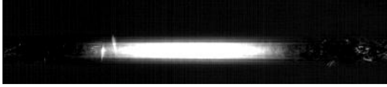
Figure 77- Relative intensity image from subtraction of 400 SLPM central jet flow from the baseline image.
