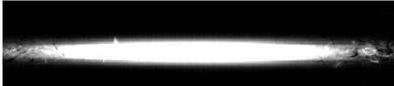
Figure 78- Relative intensity image from subtraction of 600 SLPM central jet flow from the baseline image.
